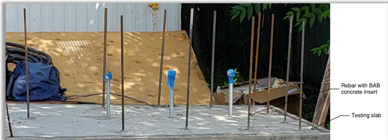
Figure 4: Test Slab for tensile and shear test
